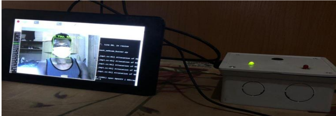
Figure 8a: The result of the human face and face mask detected.
