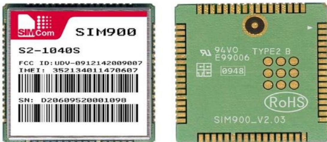
**Fig 2 SIM900 GSM/GPRS Module [1]**
